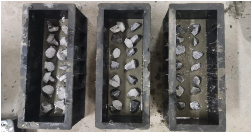
图 3 MRCAC 棱柱体浇筑 Fig 3. Prism Casting of MRCAC
