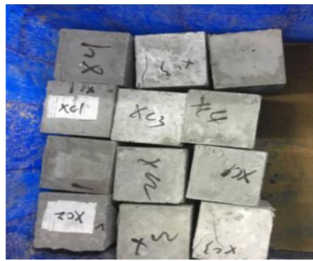
(a) Compression loading test block
