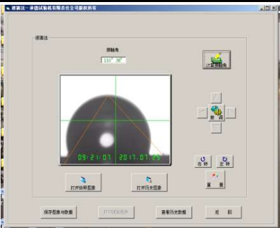
图 7 新型防污闪涂料制备涂层憎水性恢复的静态接触角 Fig. 7 Static contact angle after hydrophobicity recovery for coatings prepared with novel anti-pollution flashover coatings
