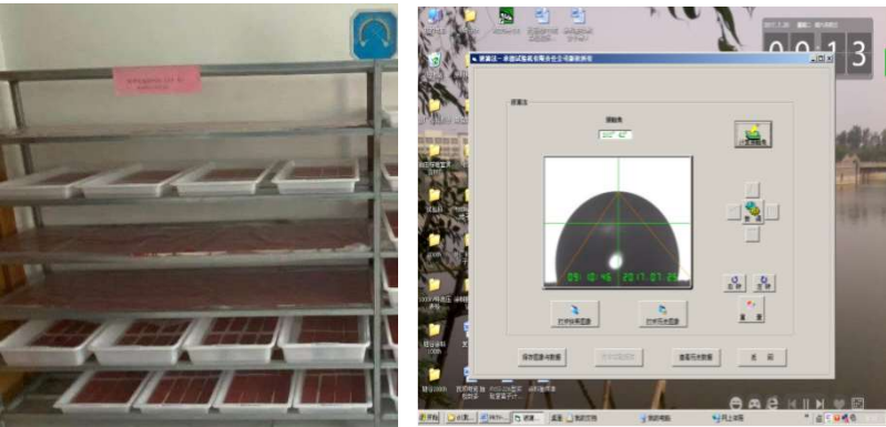
图 6 新型防污闪涂料制备涂层憎水性减弱 192h 的静态接触角 Fig. 6 Static contact angle after 192h hydrophobicity decline for coatings prepared with novel anti-pollution flashover coatings
