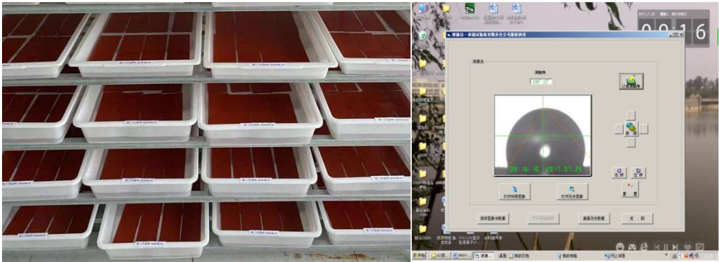
图 5 新型防污闪涂料制备涂层憎水性减弱 96h 的静态接触角 Fig. 5 Static contact angle after 96h hydrophobicity decline for coatings prepared with novel anti-pollution flashover coatings
